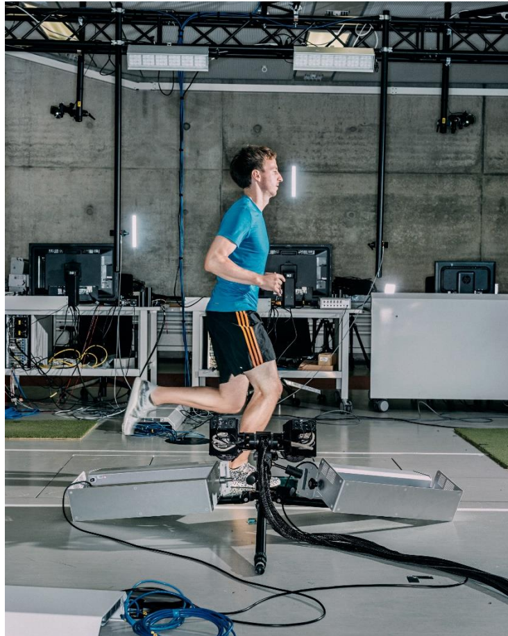
A motion-capture system collects data on an Adidas shoe. ÉRIVER HIJANO
