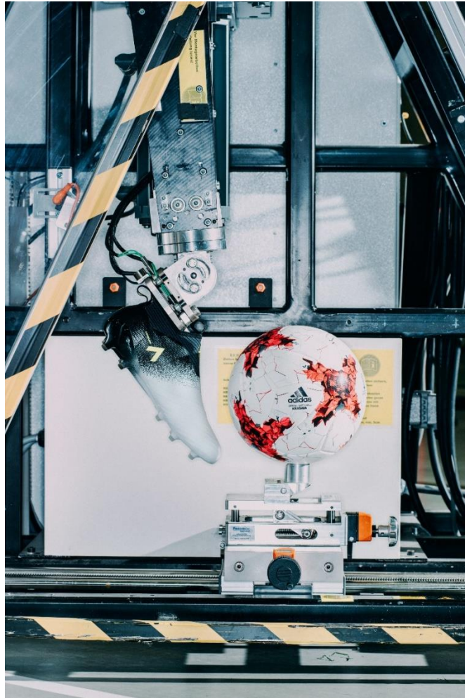
Adidas uses a ball-kicking robot to test products at its headquarters. ÉRIVER HIJANO
